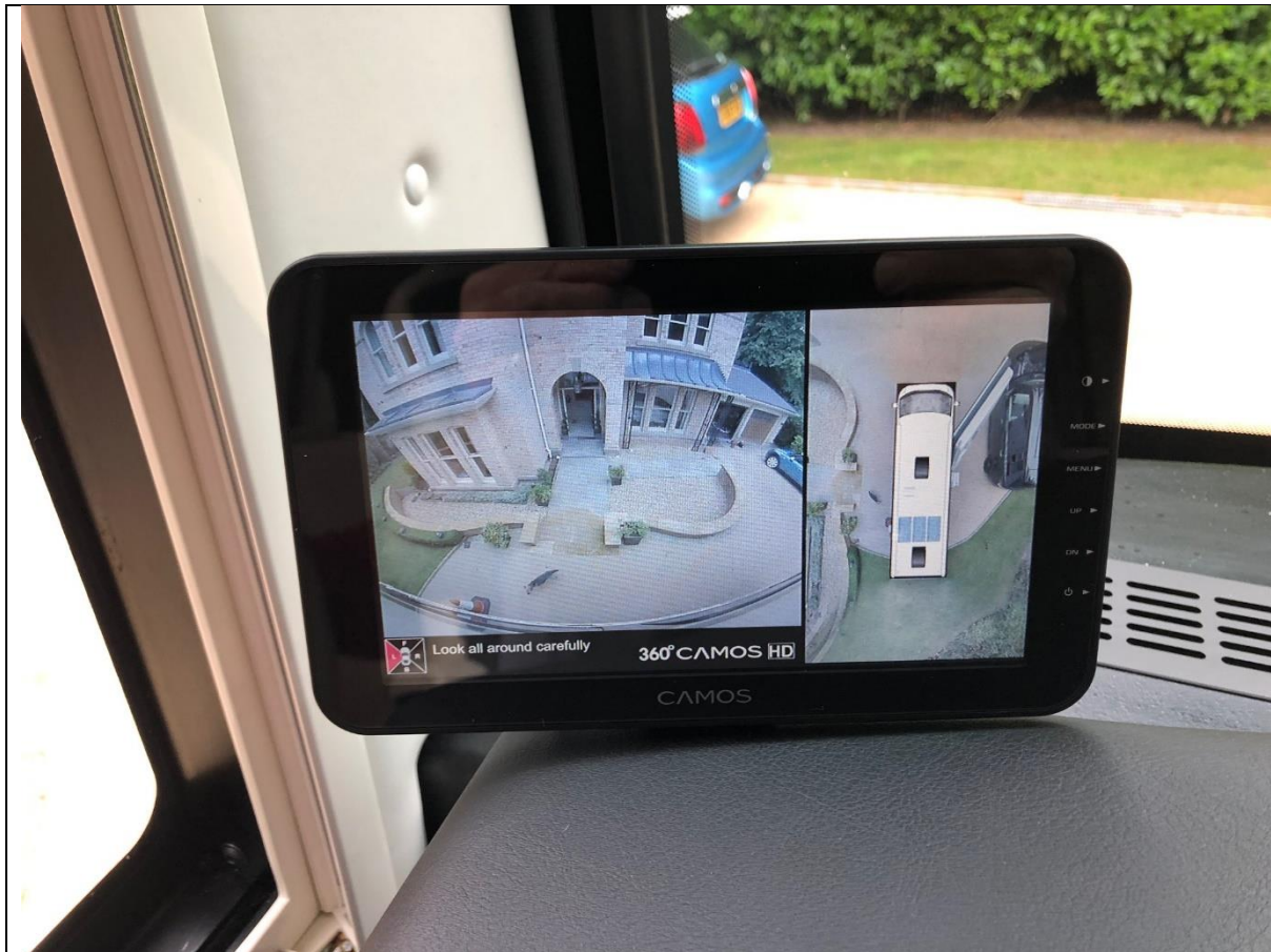
I've initiated the left indicator and the view has changed. I've chosen to have the birds eye in the right pane on all pages. So, when overtaking abroad, I indicate and you are immediately warned if there are any cars overtaking in your blind spot.
