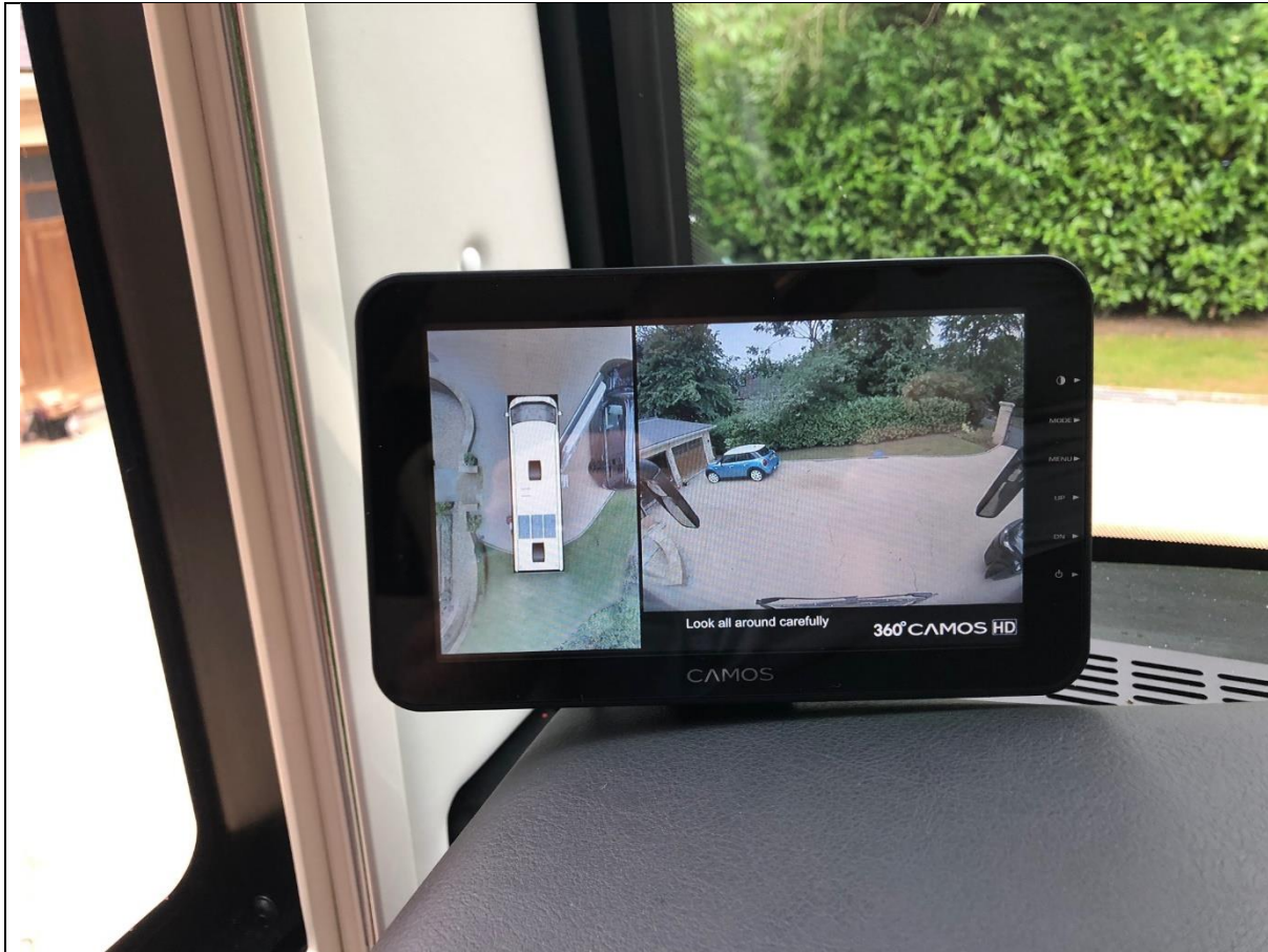
Image from set up. This shows birds eye and front view. You can see the wipers. This was not the final set up as the van outline was not correct.
