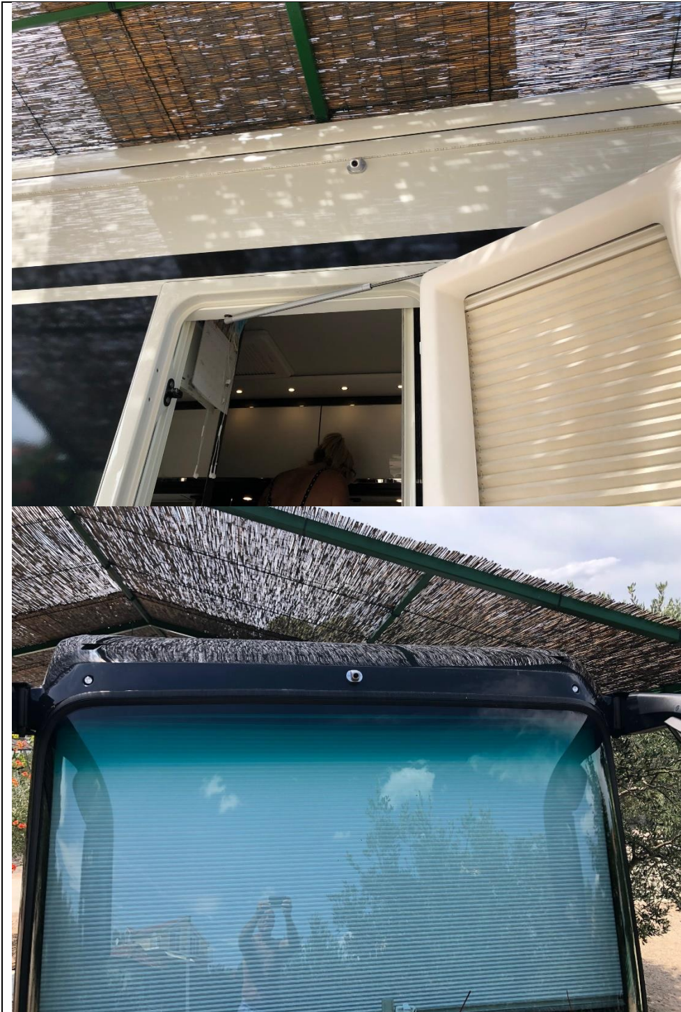
There is a 180 deg fish eye camera mounted “centrally” on each face of the van. Including the back. The images from each of the 4 caemaeras is “knitted together” by the ecu to create the birds eye view. I will get the aluminium camera bodies painted when I have some mathcing paint.
